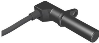
The True Position/Zero Speed sensor incorporates a DHE (Differential Hall Effect) sensor. The Hall effect gives an output when subjected to a changing magnetic field. The field is set up by a magnet inside the sensor body and changes when ferromagnetic teeth are passed beneath the sensor (no magnets are required in the target). The sensor responds to changes in magnetic field strength by corresponding to tooth frequencies down to 0Hz.
